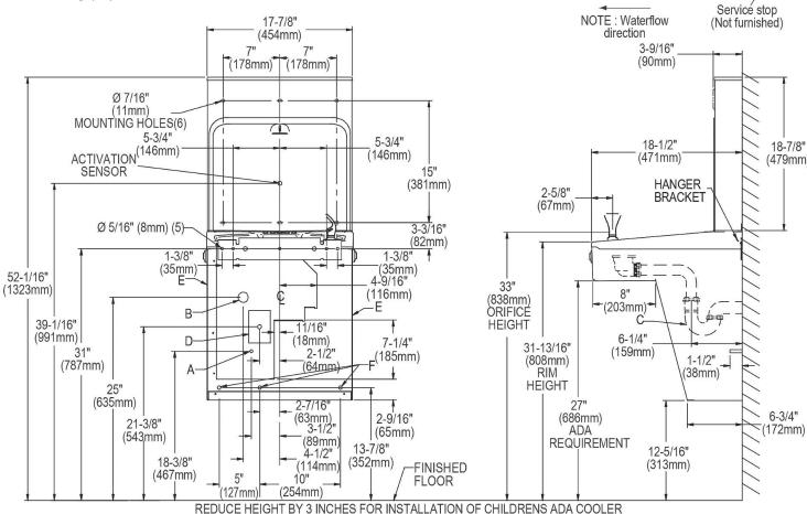
A = Recommended Water Supply location. Shut-off Valve (not furnished) to accept 3/8" O.D. unplated copper tube. Up to 3" (76mm) maximum out from wall. B = Recommended Waste Outlet location. To accommodate 1-1/4" nominal drain. Drain stub 2" (51mm) out from wall. C = 1-1/4" Trap (not furnished).
